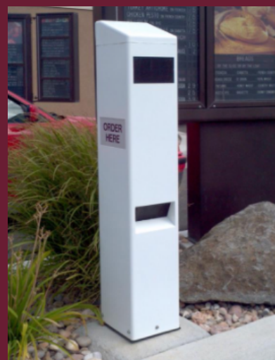
A Call Box Uses a Speaker as both a Microphone and a Speaker
